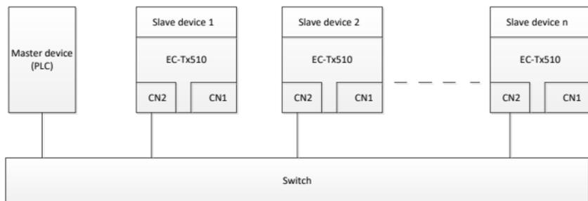
Figure 3-3 Electrical wiring diagram for a star topology
