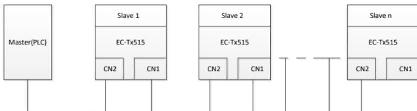
Figure 5-2 Electrical wiring diagram for a linear topology
