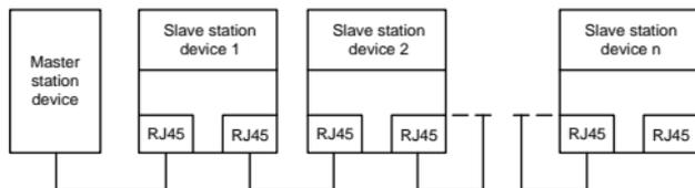
Figure 2-2 Electrical wiring diagram for a linear topology
