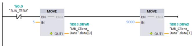
Download the PLC program to the PLC after the program has been written completely. Set VFD function codes such as P00.01=2, P00.02=0, P00.06=8, P14.00=2, P16.02–P16.05=192.168.0.2, and keep default values of P16.06–P16.13. Then, you can use the I0.0 input terminal to control the VFD to start and stop at 50.00Hz through ModbusTCP protocol.
