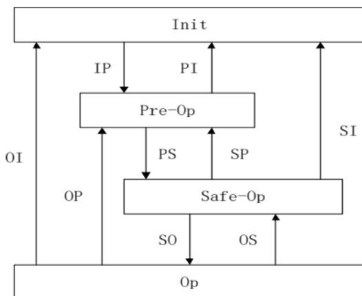
Figure 4-4 EtherCAT state machine flowchart
