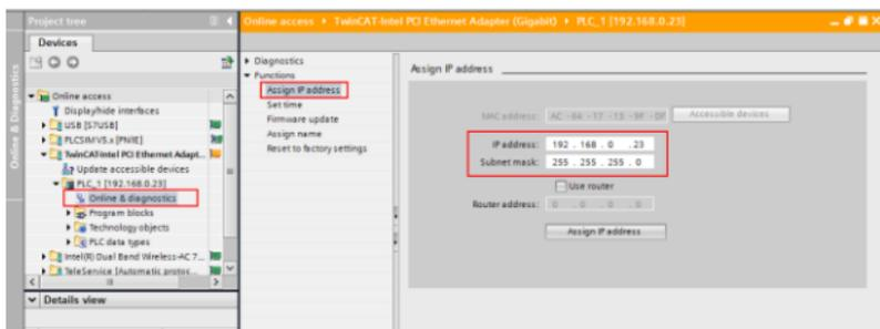
4) Set the IP address of the PLC to "192.168.0.1" and subnet mask to "255.255.255.0" (you can check "Use router", that is, the router assigns IP). Click the "Assign IP address" button after the setting is completed, as shown in the following figure.
