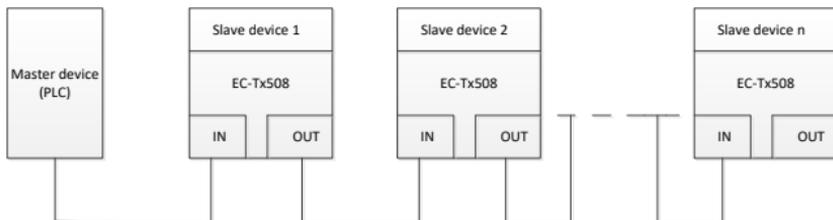
Figure 4-2 Electrical wiring diagram for a linear topology
