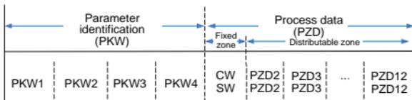
Figure 3-5 Packet structure
