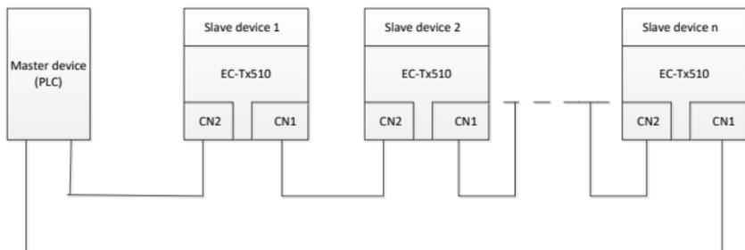
Figure 3-4 Electrical wiring diagram for a ring network
