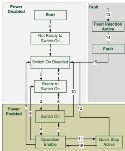
Figure 4-7 CANopen over EtherCAT state machine
