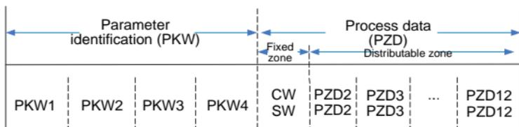
Figure 2-4 Packet structure
