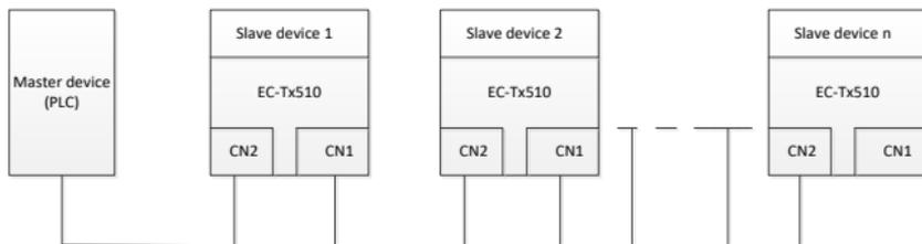
Figure 3-2 Electrical wiring diagram for a linear topology
