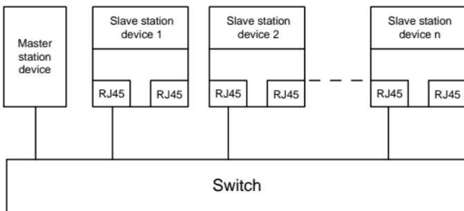
Figure 2-3 Electrical wiring diagram for a star topology
