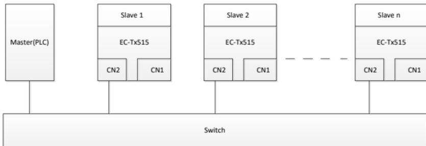
Figure 5-3 Electrical wiring diagram for a star topology
