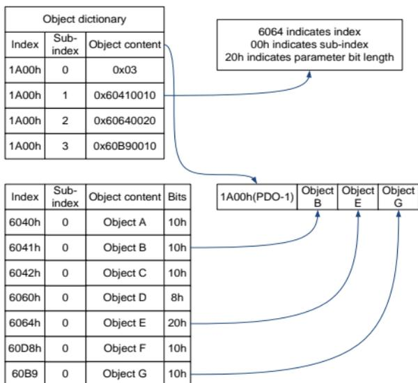
Figure 4-5 PDO mapping method
